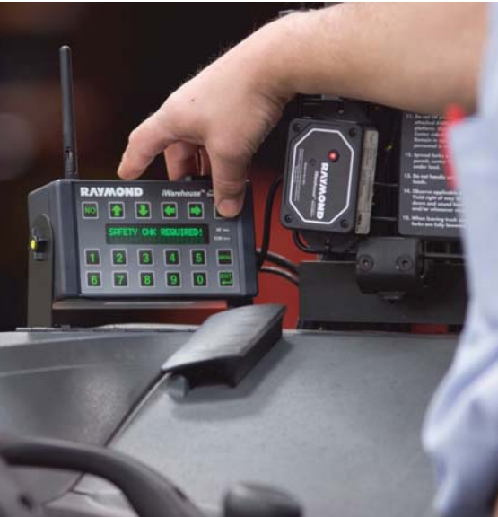
▲ Raymond Corp.'s iWarehouse system allows warehouse and distribution managers to collect and analyze real-time truck data.
