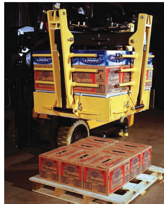
▲ Tygard Machine & Manufacturing Co. supplies a side-mount claw, which can pick nearly 2,000 cases per hour.
