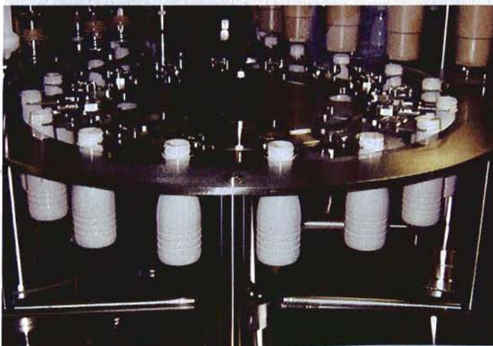
BUNDLING, FILLING. Filled, capped, and labeled bottles are funneled into four lanes ahead of the shrink bundler. Photo below shows bottles moving from filler to capper.
