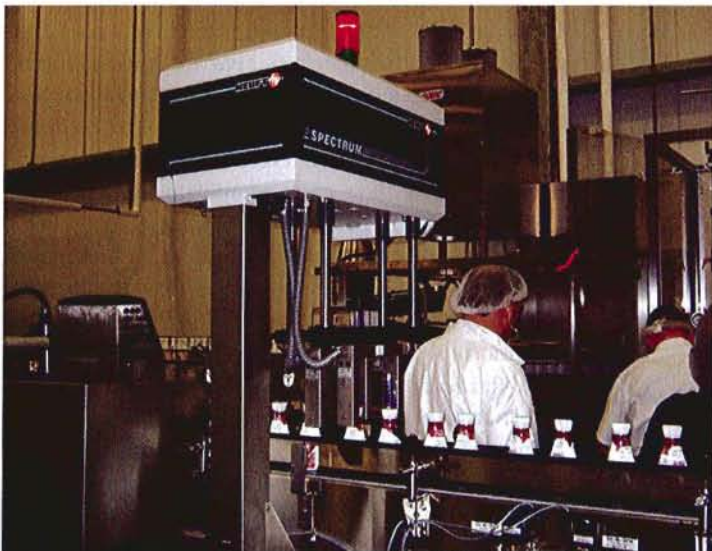
INSPECTION SYSTEM. Capping torque, cap position, and fill height are all checked automatically by this high-speed inspection system.
