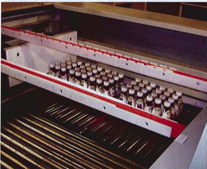
OVERHEAD PALLETIZER. The overhead palletizer collates shrink-bundled bottles in the desired pattern and then pushes them smoothly onto pallets.
